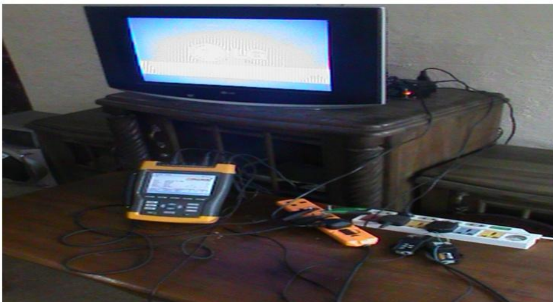
Plate B4: Acquisition and Analysis of Supplied Power Signal for TV by FLUKE 435
