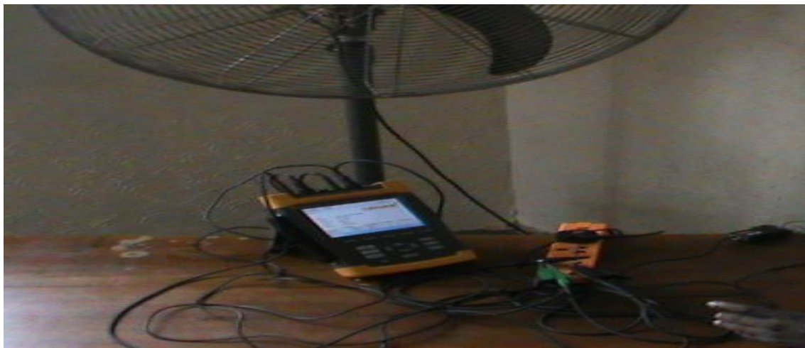
Plate B3: Acquisition and Analysis of Supplied Power Signal for Fan by FLUKE 435
