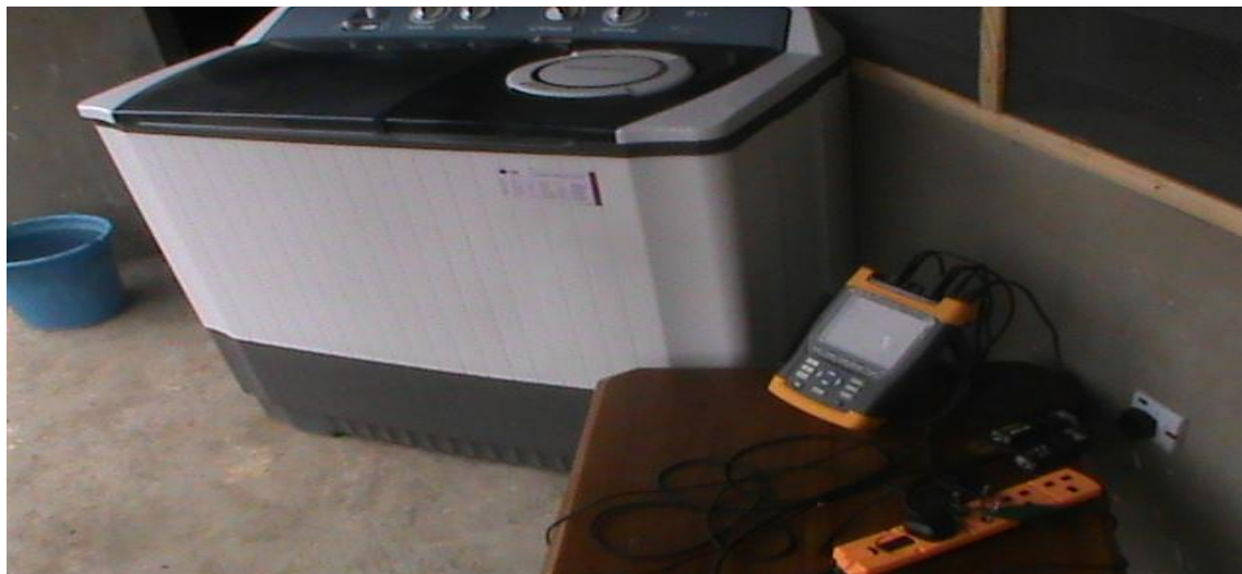
Plate B5: Acquisition and Analysis of Supplied Power Signal for Washing Machine by FLUKE 435
