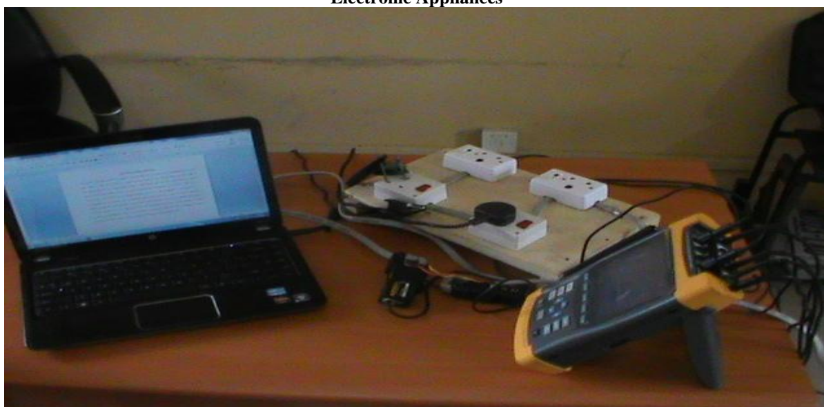
Plate B1: Acquisition and Analysis of Supplied Power Signal for Laptop by FLUKE 435
