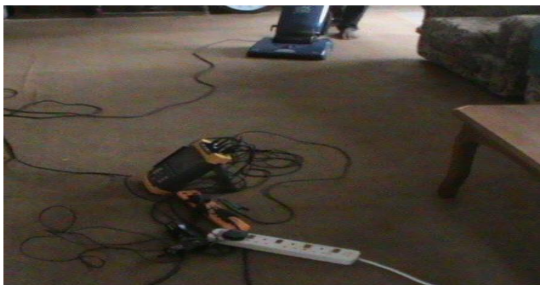
Plate B6: Acquisition and Analysis of Supplied Power Signal for Vacuum Cleaner by FLUKE 435
